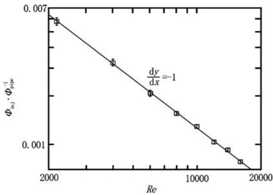
Fig.3 Experimental results for pipe flow: the normalized flow rate of disturbance versus the Reynolds number (Hof, Juel, and Mullin [10]). The range of Re is from 2000 to 18,000. The normalized flow rate of disturbance is equivalent to the normalized amplitude of disturbance for the scaling of Reynolds number,  $\Phi_{inj} / \Phi_{pipe} \sim (v'_m / U)_c$
