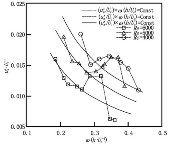
Fig. 6 Variation of critical amplitude of disturbance velocity,  $u'_m / U_c$ , against the disturbance frequency  $\omega(h / U_c)$ . Comparison of the present theory Eq.(10) with the experimental data in [20]. Here,  $h$  is the half channel width,  $\omega$  is the angular frequency of disturbance,  $U_c$  is the centreline velocity, and  $u'_m$  is the disturbance amplitude of streamwise velocity
