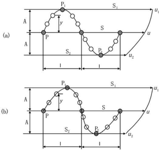
Fig.2 Movement of a particle around its original equilibrium position in a cycle of disturbance. (a) Ideal case; (b) Wave deformed
