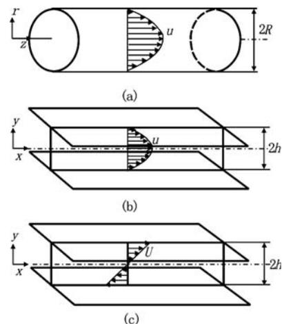
Fig.1 Schematic of wall bounded parallel flows. (a) Pipe Poiseuille flow; (b) Plane Poiseuille flow; (c) Plane Couette flow
