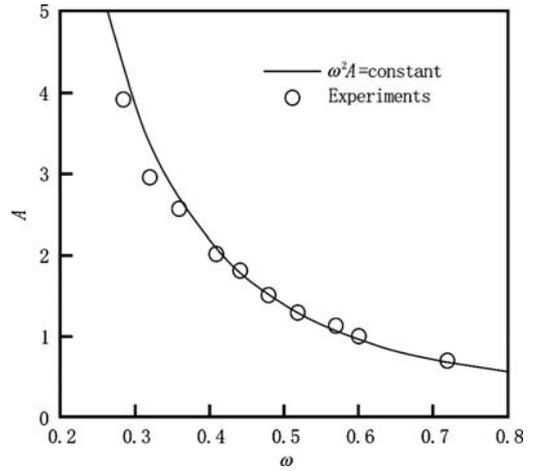
Fig. 5 Variation of critical disturbance amplitude,  $A$ , against the driving angular frequency  $\omega$  at  $Re=2200$  for the single-jet disturbance. Comparison of the present theory Eq.(10) with the experimental data in [9]
